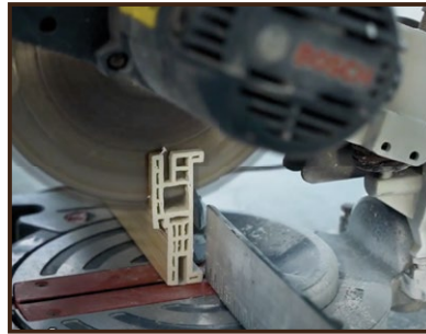
Bước 2: Cắt 2 gờ khung bao đúng Step 2: Cut the vertical frame edges as the technique drawing.
